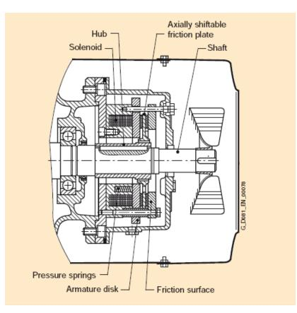
The electro-magnet (solenoid) two-surface KFB spring-operated disk brake is a safety brake. When the current is disconnected, the armature disk and the support for the friction pads are pressed against the mating frictional surface. This is what causes the braking effect.
