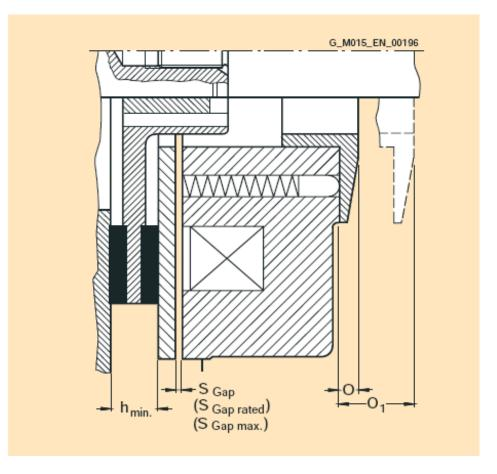
When in the no-current condition, the brake is electromagnetically released. When braking operation starts, the rotor - that can axially move along the shaft - is pressed onto the mating frictional surfaces using springs that act on the armature disk. In the braked state there is a defined air gap between the armature disk and the solenoid assembly. This air gap can increase as the brake pads wear.
